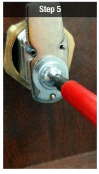
Install screw on top of round washer and tighten
