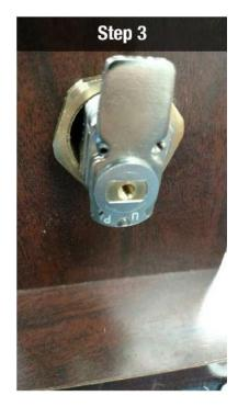
Install the Rotation Control Plate as shown.
